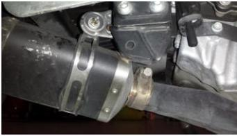
**NOTE:** The adapter has been sprayed with WD-40 to keep it from rusting. It should be clean before welding not to contaminate the weld.
