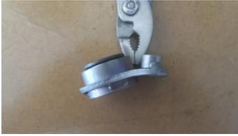
Then remove the top 6mm bolt and loosen up the bottom one to let the hanger pivot down and meet with the exhaust strap. Once all attach together make sure everything is all tight. Not using the exhaust strap might end up breaking the slip-on on the inlet side due to excessive vibrations. (Sorry for the dirtiness, haven't clean my bike in a while 😊 )
