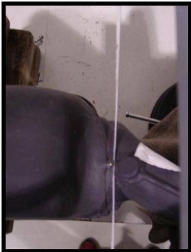
First step is to remove your exhaust system from your motorcycle. Once it is off the motorcycle, you can hold the headers in a vise for the cutting part. Using a rag to put around the primary pipe will avoid damage.
