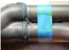
2. Using masking or electrical tape, mark your cutting line. 1/2" to 3/4" from the weld should be good. You need to keep the primary pipe as long as possible and make sure you cut all the weld so the tubes are free of weld. Look between the tubes and cut to leave as much material as possible.
