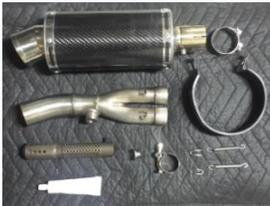
Before starting your installation and looking at your parts, you will notice the 2 spring hooks. If you prefer using those instead of the hook clamp you should slip the collector over the headers and bring the hook and springs to a welder. 1/4" preload on the springs is sufficient. Hooks and collector are 304 stainless steel.
