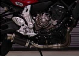
5. Once the collector on the headers you can go ahead and install the headers on your motorcycle. Make sure the exhaust gaskets stays in place. Few drip of silicone will hold them in place. You can also install your O2 sensor. You can either use a M18 Wideband sensor or the OEM M12 sensor with the adaptor supply in the kit. Leave the 4 flange nut just a bit loose to be able to move them around for best fit possible.
