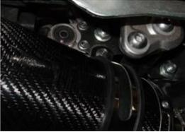
6. You can now install the Exhaust strap/rubber to support your Delkevic slip-on. Remove the 8mm nut from the OEM exhaust and reuse the bolt. (You can remove the OEM exhaust support hanger) and attach the exhaust strap to the chassis as shown on the picture (add one washer on each side provided in the kit). Now you can move your exhaust around and until it find it's happy place, then tighten every single nut & bolt to Yamaha specs.
