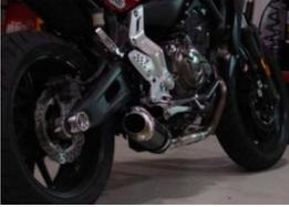
Install the Delkevic slip-on with the DBK installed. Aim the slip-on so have enough clearance all around.
