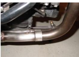
4. You are now ready to slip the tube in the collector. You can apply some high temp silicone (provided in the kit) in the collector side to seal the headers pipe in the collector. If you are using the clamp adaptor for the spring, insert it before you slip the tube on the collector. Clamp goes on the LH tube.
