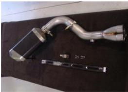
9. Go over all the hardware and make sure everything is all nice and tight. Double check for exhaust leak between the headers and engine. Do not over tight the exhaust clamp.
