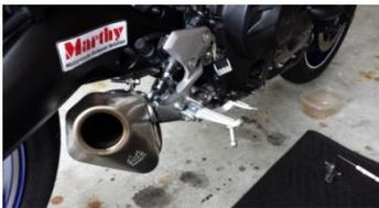
8. Aim the slip-on so it doesn't interfere with the swing arm, rear set or tire. Going up and down with the mid-pipe and rotating the slip-on should give you plenty of room for a perfect fit. There's some room too on the mid pipe, doesn't have to go all the way in. Install the slip-on strap with the other long bolt. There's a white protecting film that you need to peel off on the exhaust strap.
