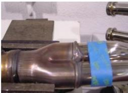
2. Using masking or electrical tape, mark your cutting line. 3/8" to 1/2" from the weld should be good. You need to keep the primary pipe as long as possible and make sure you cut all the weld so the tubes are free of weld. Look around in each 3 spaces and cut to leave as much material as possible.
