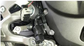
7. Install the provided support bracket (short end goes on the bike) When this is all done you can install your mid pipe, slip-on assembly.
