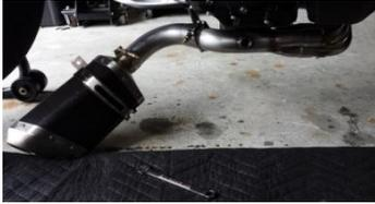
6. You can now pre assembly your slip-on and mid pipe with the exhaust clamp in place. Leave everything snug only. That will permit you to adjust the slip-on to the perfect location. Use the 2 long bolts that support the OEM exhaust. Pry the little tab on your stock exhaust to remove the nuts.
