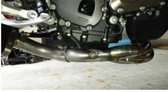
5. Once the collector on the headers you can go ahead and install the headers on your motorcycle. Make sure the exhaust gaskets stays in place. Few drip of high temp silicone will hold them in place. You can also install your O2 sensor and attach the 2 springs.
