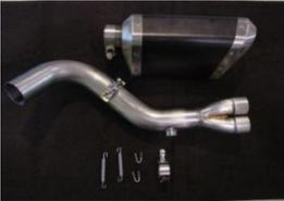
Before starting your installation and looking at your parts, you will notice the 2 spring hooks. If you prefer using those instead of the hook clamp you should slip the collector over the headers and bring the hook and springs to a welder. 1/4" preload on the springs is sufficient. Hooks and collector are 304 stainless steel.
